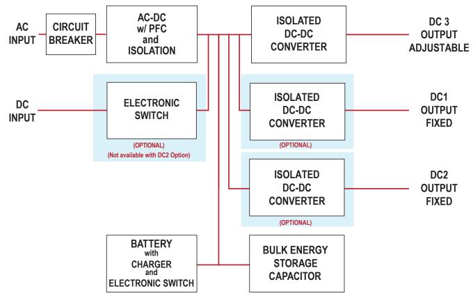
Power flows from the AC INPUT through an AC-DC converter that has Power Factor Correction (PFC) and high voltage safety isolation. Power flows from the DC INPUT through an electronic switch that is closed when the AC INPUT power is absent and the DC INPUT voltage is within its specified range. Otherwise, a second electronic switch is closed to connect the battery to the mid-bus.
